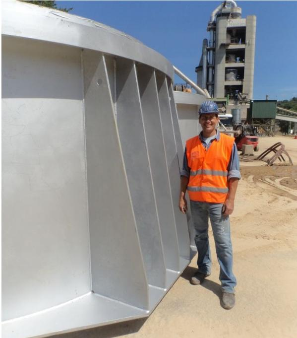
The latest modification applies the replacement of four cyclones and all appropriate input and output ducts to the raw mill and was realised in 2015. The result was a reduction of dust by 66%, a reduced power consumption and a low pressure drop of the cyclones (6,1 mbar) as well as an excellent separation efficiency of 95%.
