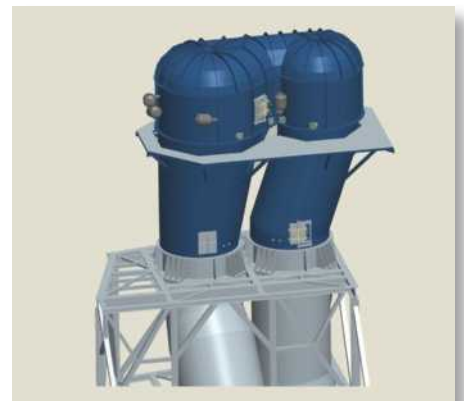
Figure 4: Specific design of the A TEC Post Combustion Chamber (PCC)
