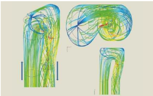
Figure 7: CFD analysis of the gas flow in the calciner loop of the post combustion chamber
