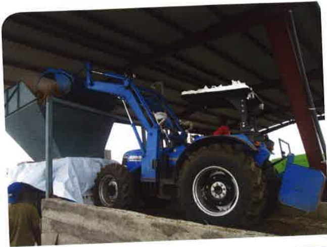
Figure 2. Feeding the biomass into the baler.
