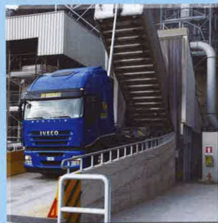
"TIRES" - Receiver from trucks and feeder for several bulk materials
