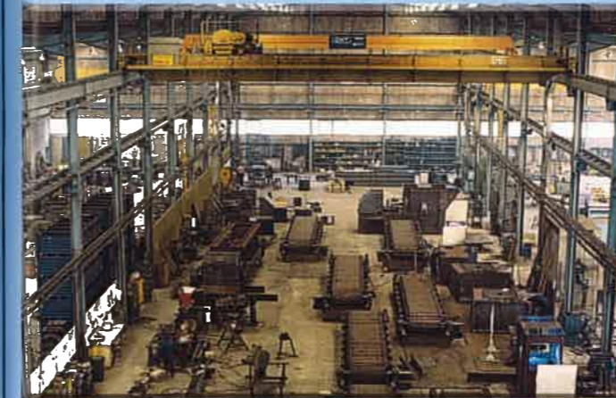
Apron feeders for clinker and limestone - Preassembly in our work shop
