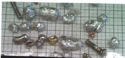
Figure 14: inorganic material collected at the ROCKET MILL's slide gates during operation
